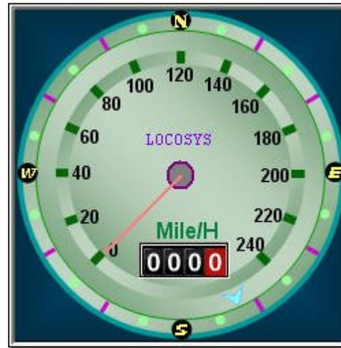
The **COG&SOG View** displays the GPS speed and direction in a graphical form. There are two measurement systems can be shown: Metric (KM) or Imperial (Mile). You can select the unit of measurement in the Unit selection box on **Function Bar** by click the item of KM or Mile.
