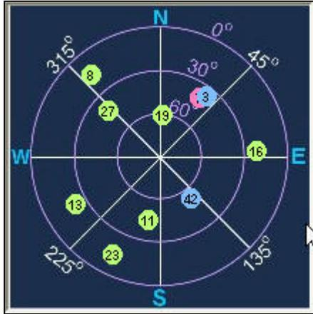
The **Radar View** displays the azimuth and elevation of tracked and available satellites in a graphical form. The color of the satellite status is:
